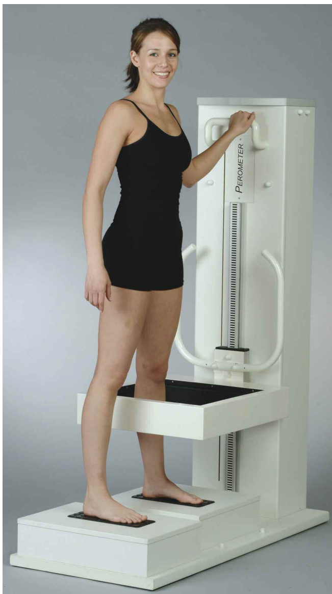
Most often used in research settings, the Perometer® uses infrared beams to scan the girth of a limb. Courtesy Julius Zorn, Inc.
